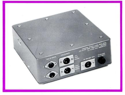
Cartridge impedance interaction effects are exceptionally low and the harmonic distortion at all audio frequencies, at normal signal levels, is below the noise. The amplifier has very low levels of static and dynamic intermodulation distortion and low hum levels are achieved by the use of an electrostatically screened and mumetal shrouded mains transformer. Precautions are taken in the input stages to minimise radio frequency interference.
